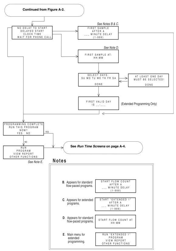
Figure A-3 Standard and Extended Programming: Start Times
