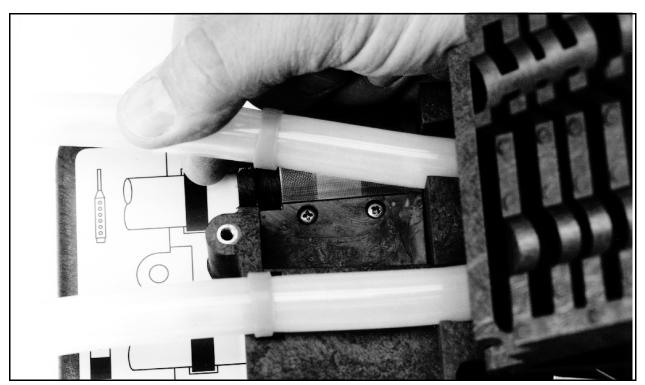
Figure 7-2 Placing the Pump Tube in the Liquid Detector
