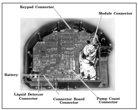
Figure 7-4 Main Circuit Board Connections
