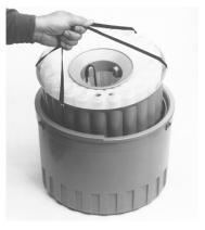
Removing Bottles From the Compact Sampler
