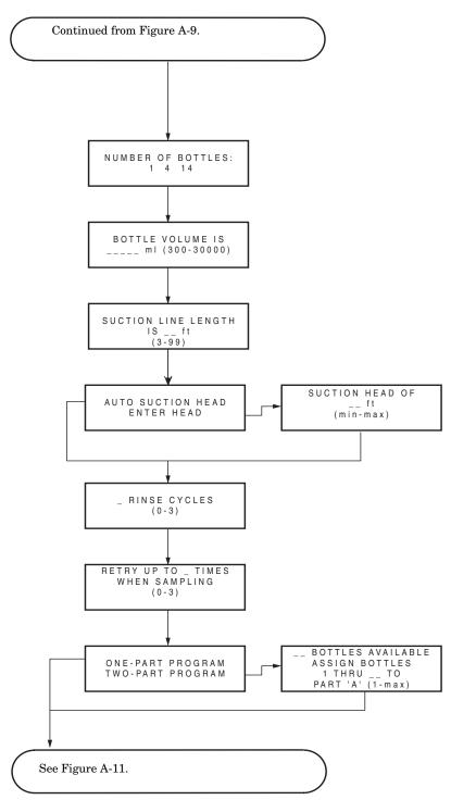
Figure A-10 Extended Programming: Equipment Setup
