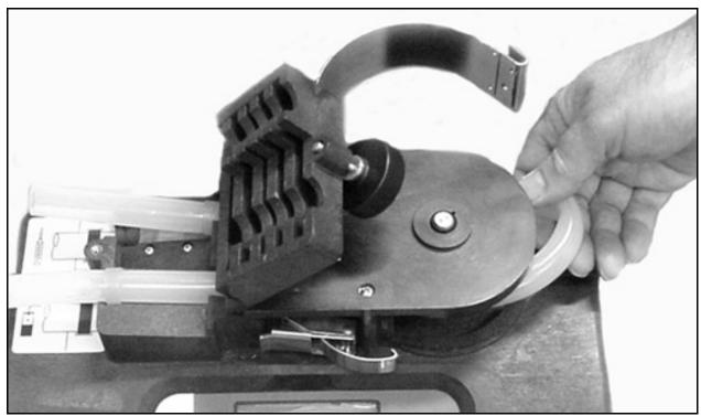
Figure 7-1 Removing and Replacing the Pump Tube
