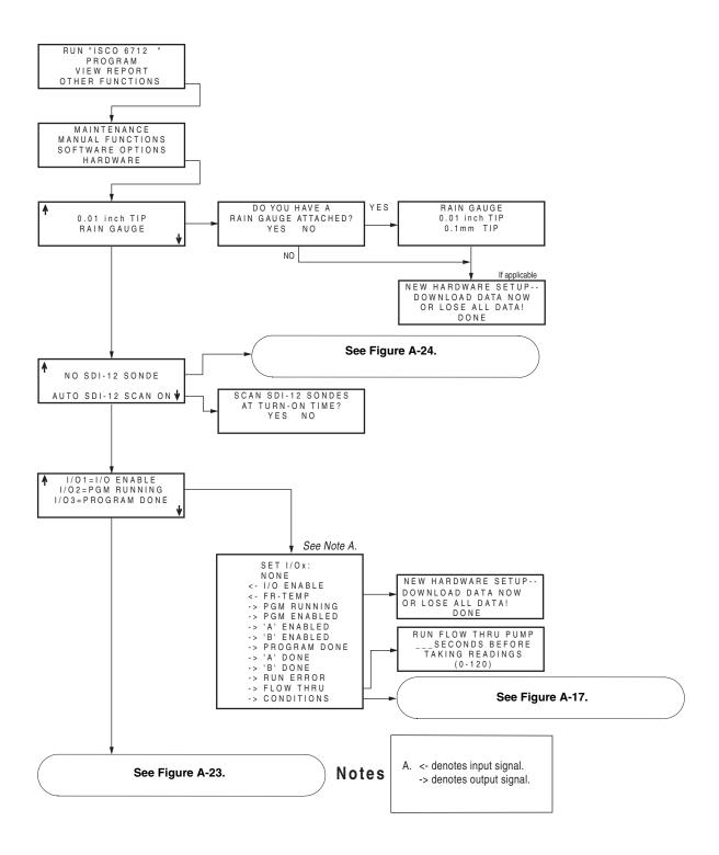
Figure A-21 Extended Programming: Quick View; Hardware
