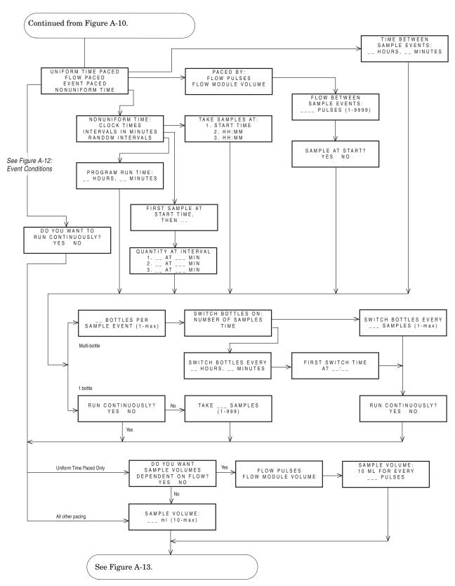
Figure A-11 Extended Programming: Pacing and Distribution
