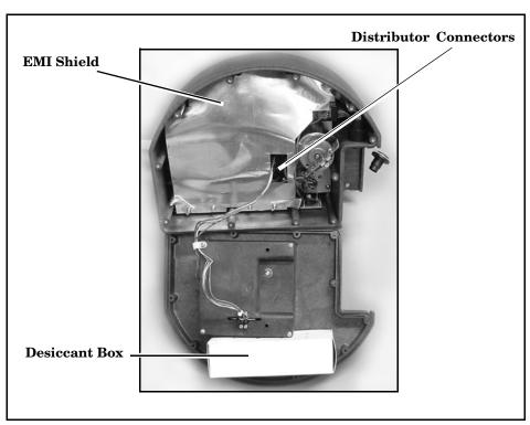
Figure 7-3 Opening the Controller
