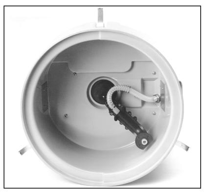
Figure 2-1 Installing the Distributor Arm
