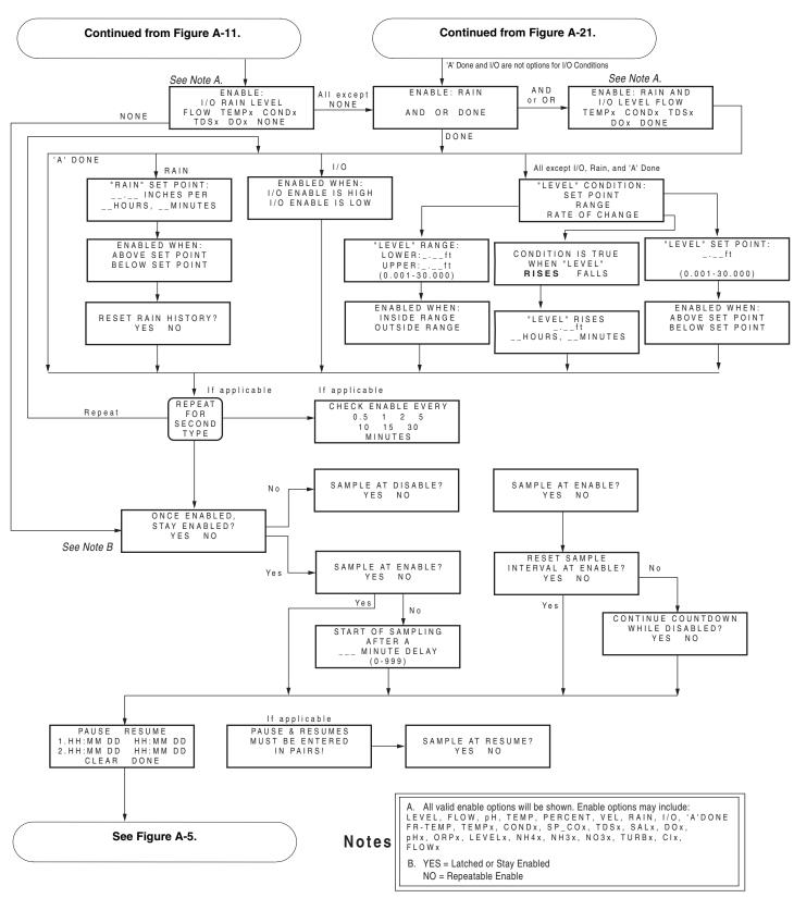
Figure A-13 Extended Programming: Programmed Sampler Enable
