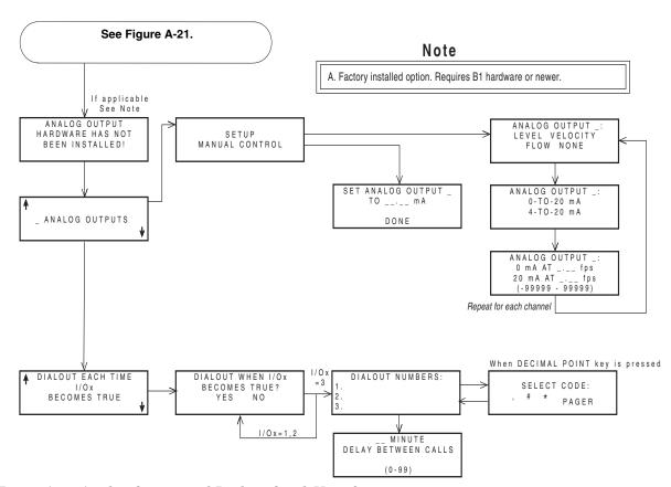
Figure A-23 Analog Output and Dialout Quick View Screens
