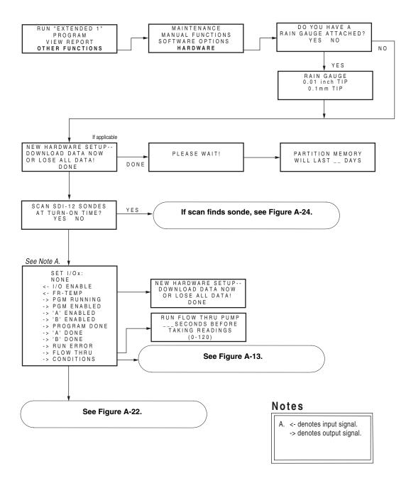
Figure A-20 Extended Programming: Normal View; Hardware
