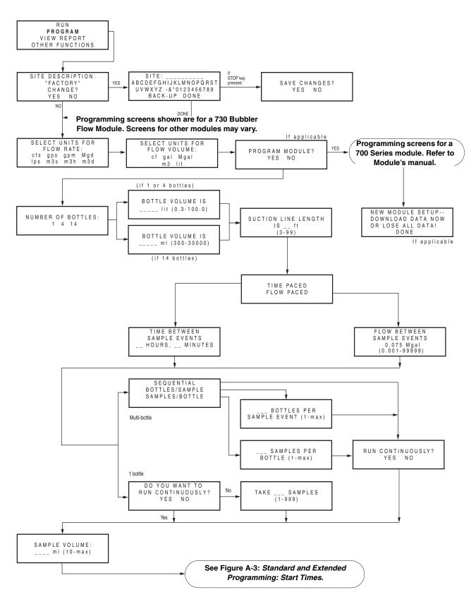
Figure A-2 Standard Programming: Programming Screens
