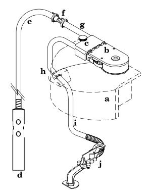
Figure 2-9 Identifying the Sampler Components
