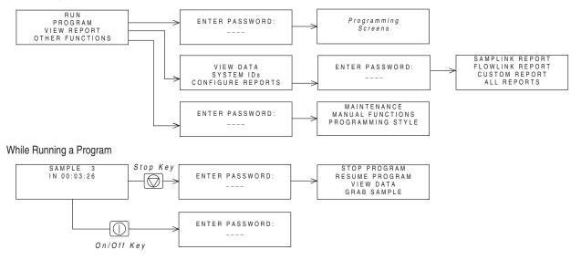
Figure 5-6 Password Protected Functions
