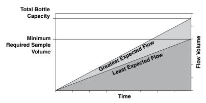
Figure 5-2 Factors Affecting Flow-Weighted Variable-Volume Samples
